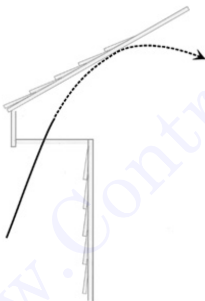
Figure 6.32 Method of drilling a hole through boxing by using a flexible shaft.
