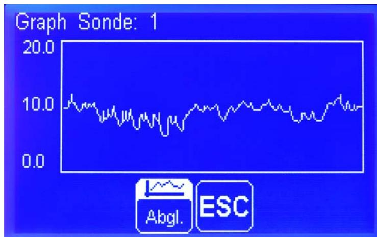
If you press the button **Cal.** at this point, the BTS-5000 will show the calibration curve for the corresponding sensor.
